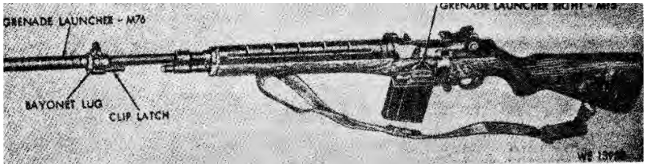
Figure 1-5. 7.62-MM Rifle ,M14 and accessories.
