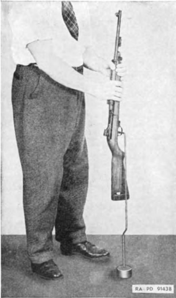
*Figure 10. Testing Trigger pull.*
