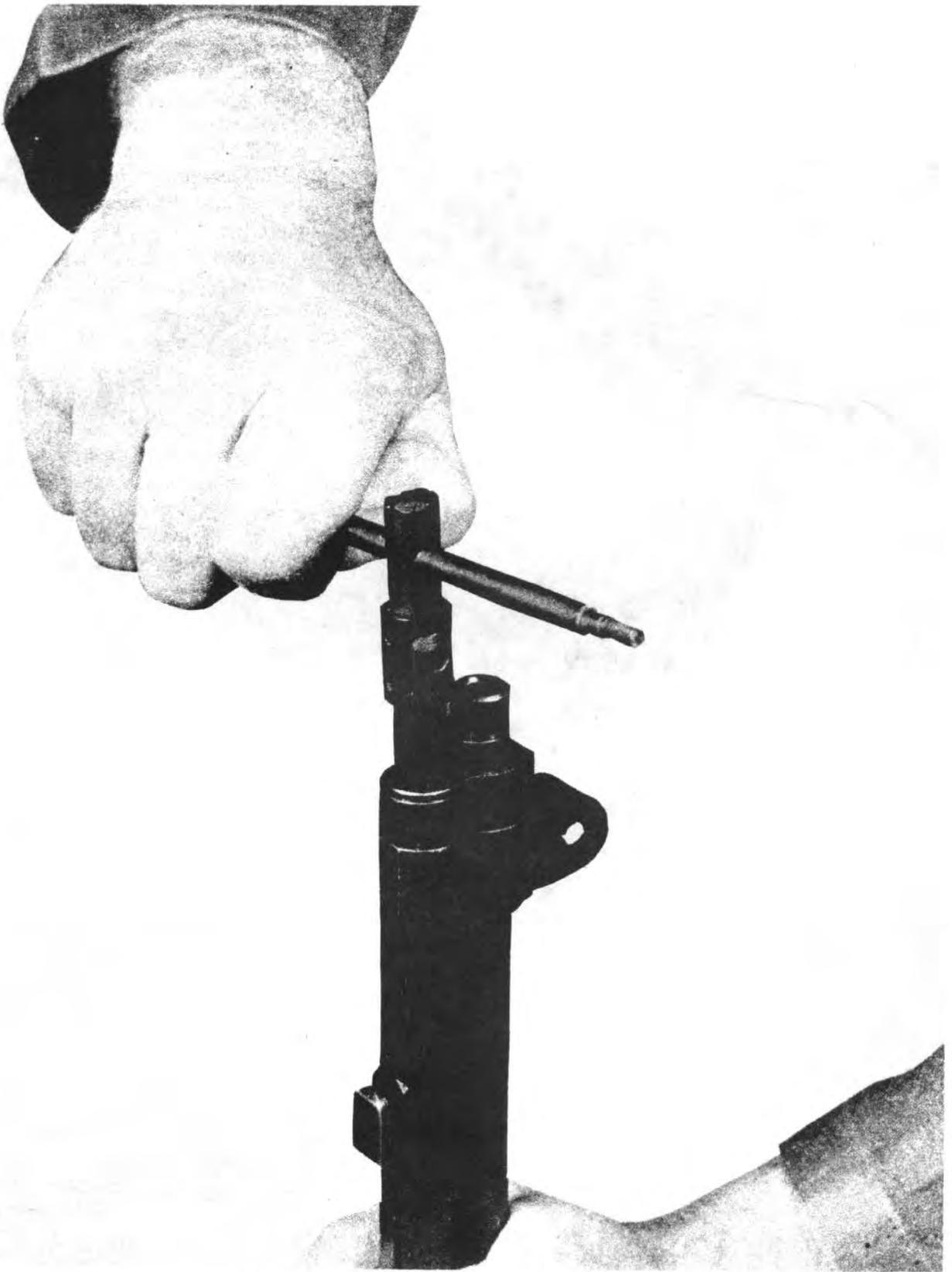
*Figure 8. Removing the gas cylinder lock screw.*
