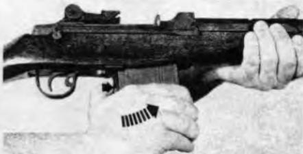
Figure 4. Removing the magazine.
