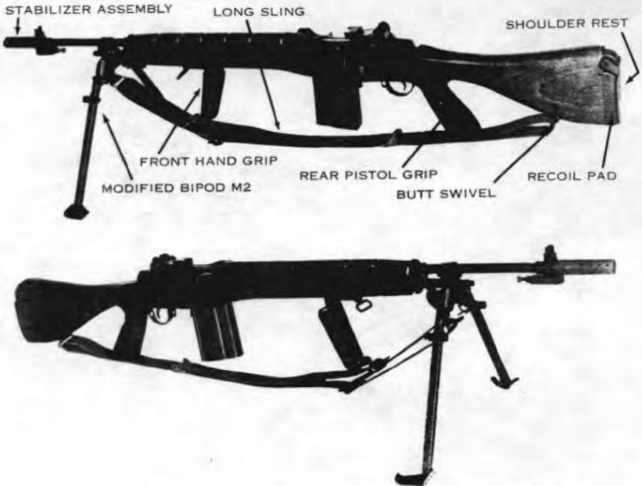
Figure 3. The M14E2 rifle (top—left side view; bottom—right side view).
