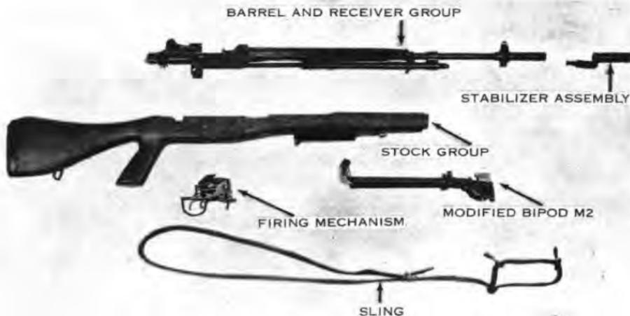
Figure 8. Components of the M14E2 rifle.
